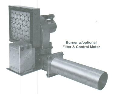
The Eclipse Extended Nozzle Minimatic burner is a compact packaged gas burner designed for firing rates up to 500,000 Btu/hr. It is used in process air heating applications, such as ovens and dryers. Minimatic burners feature an integral air and gas butterfly mounted on the same shaft for ease of set-up and dependable operation.
